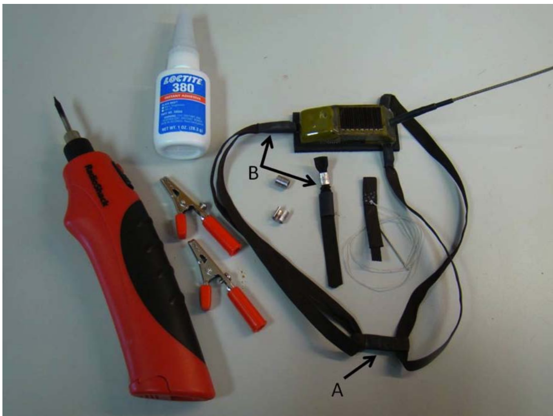
Fig. 1. Teflon ribbon harness attached to a 22 g solar-powered PTT, highlighting the belly connecting strap (A) and the connection of the harness to the front PTT ring (B).
